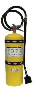
The Amerex "soft flow" extension applicator is particularly suited for fighting Class D fires. It allows the operator to stand away from the extreme heat and toxic fumes caused by burning material. The easily controlled, even discharge provides a non-dispersing application of the agent. The extension applicator may be quickly detached to provide a straight stream of chemical where greater range is required.
